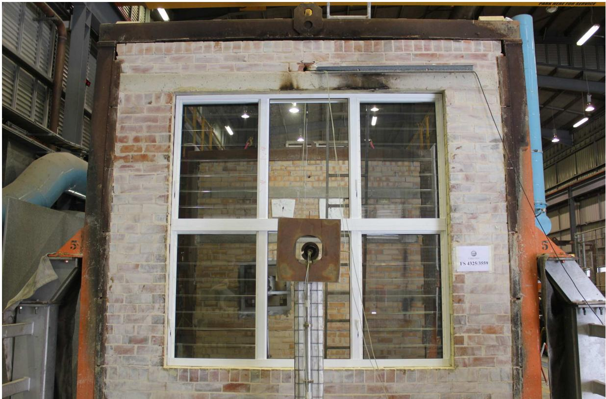
Photograph 6 - Unexposed face of the specimen at the completion of testing
