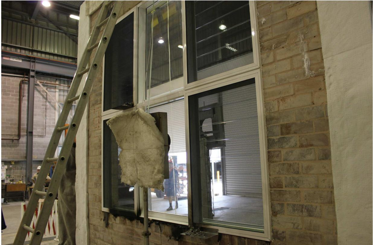
Photograph 5 - Exposed face of the specimen at 17 minutes into the test
