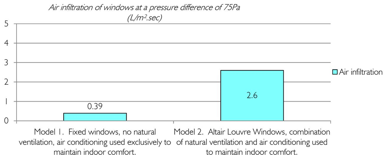
Note: The air infiltration of the fixed window is the average air infiltration rating sourced from [www.wers.net](http://www.wers.net) of 9 different fixed windows from 4 different manufacturers,
